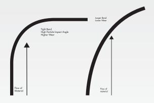
To increase the service life of hose used in a bend; it is recommended that the hose be rotated around it's axis so that the wear is more evenly distributed.
