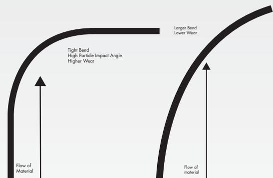
To increase the service life of hose used in a bend; it is recommended that the hose be rotated around its axis so that the wear is more evenly distributed.
